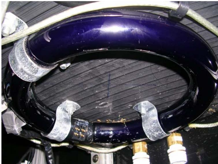
*Figure 13: FC8T9 Circline UV Fluorescent Tube*
