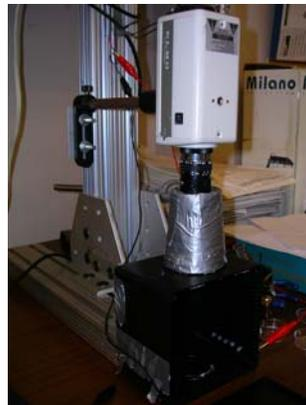
*Figure 6: Black box prototype with ELMO camera*
