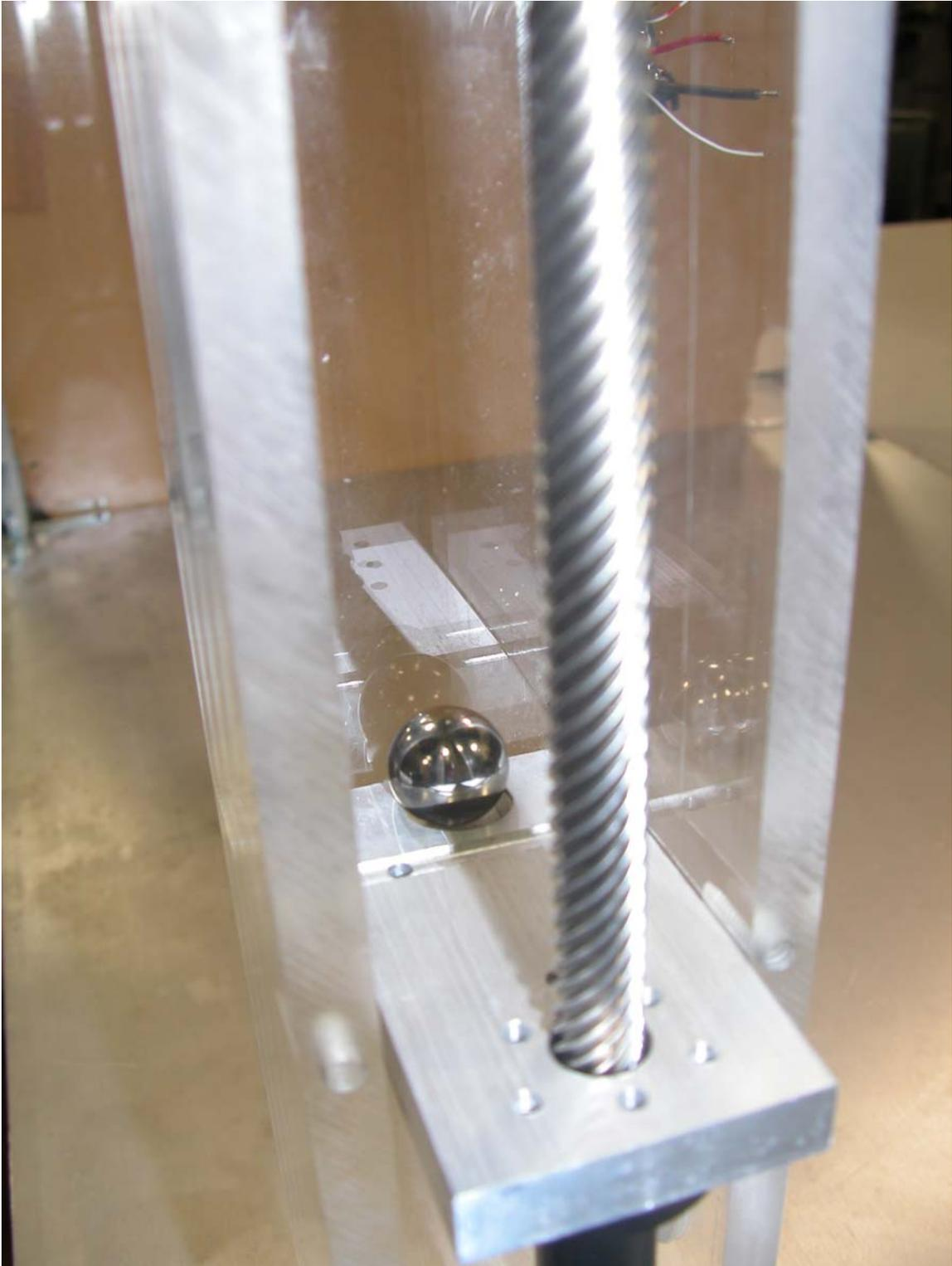
**Figure 3 – A close up of the finished elevator car in the elevator shaft with the lead screw. This view shows all parts of the elevator: car, screw, shaft and ball at the front.**
