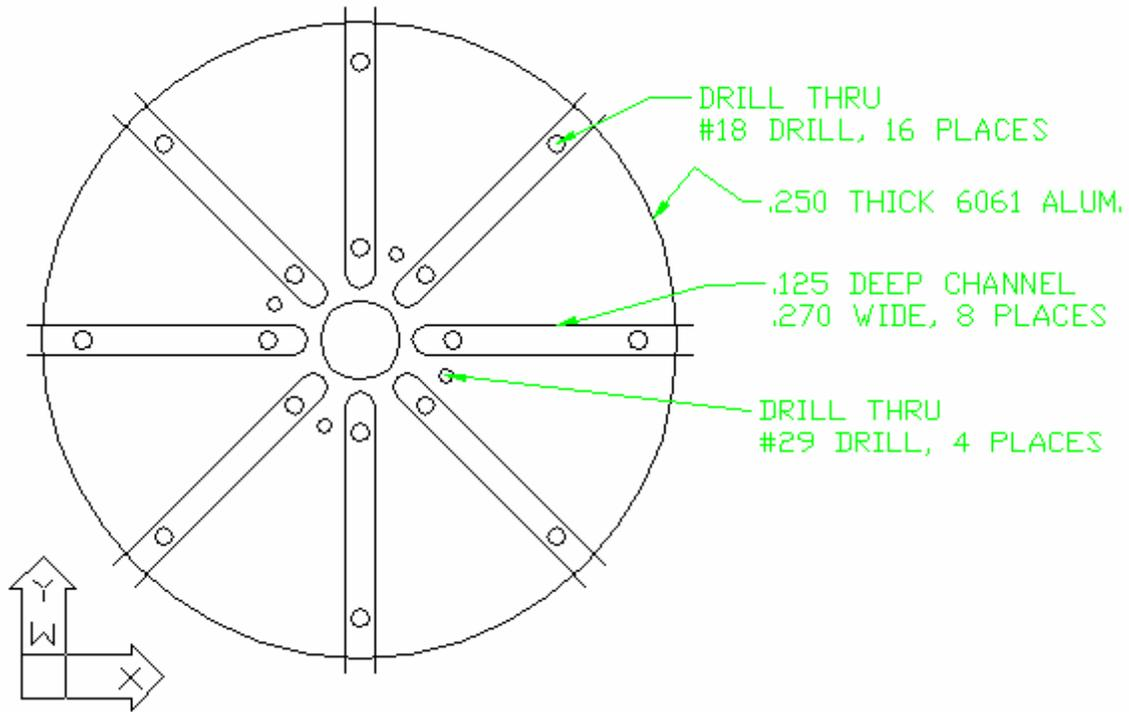
**Figure 4 – Commented CNC drawing for the side plate of the turnstile**
