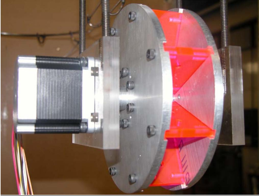
**Figure 5 – The completed turnstile, including stepper motor, hanging from the support tubing in the sculpture by  $\frac{1}{4}$  - 20 threaded rod.**
