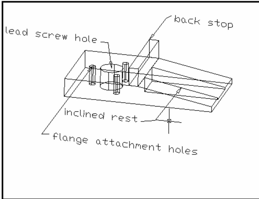
**Figure 2 – A wire frame drawing of the elevator car that moves the ball in the elevator. The car is what carries the ball up the shaft of the elevator and pushes the ball onto the track.**
