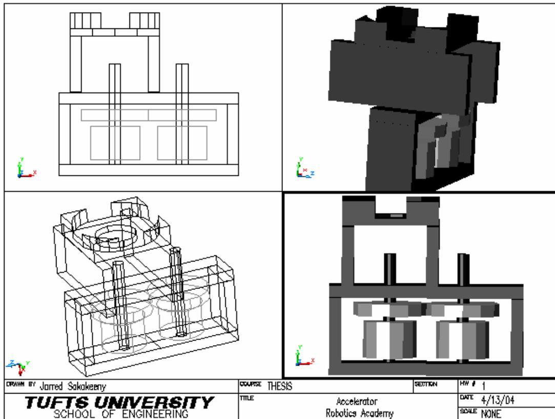
Fig 7- 3-D wire frame and Flat shaded view of the accelerator and motor mount
