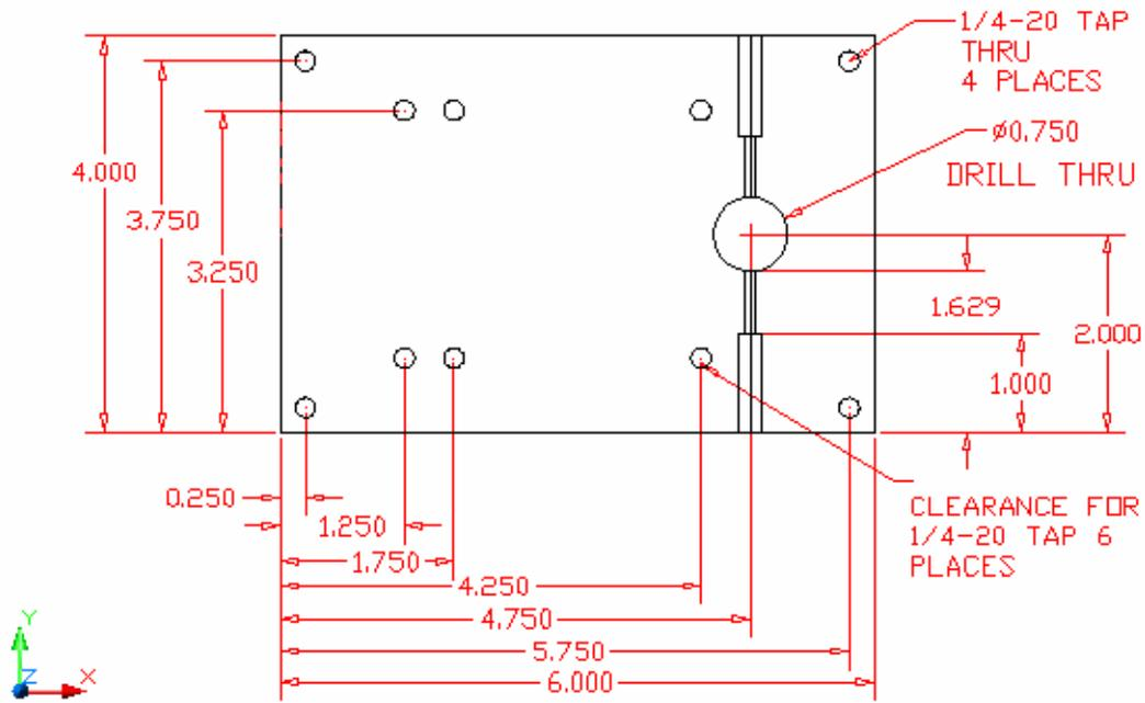
**Figure 2 – Machining drawing for the top and bottom plates of the elevator.**
