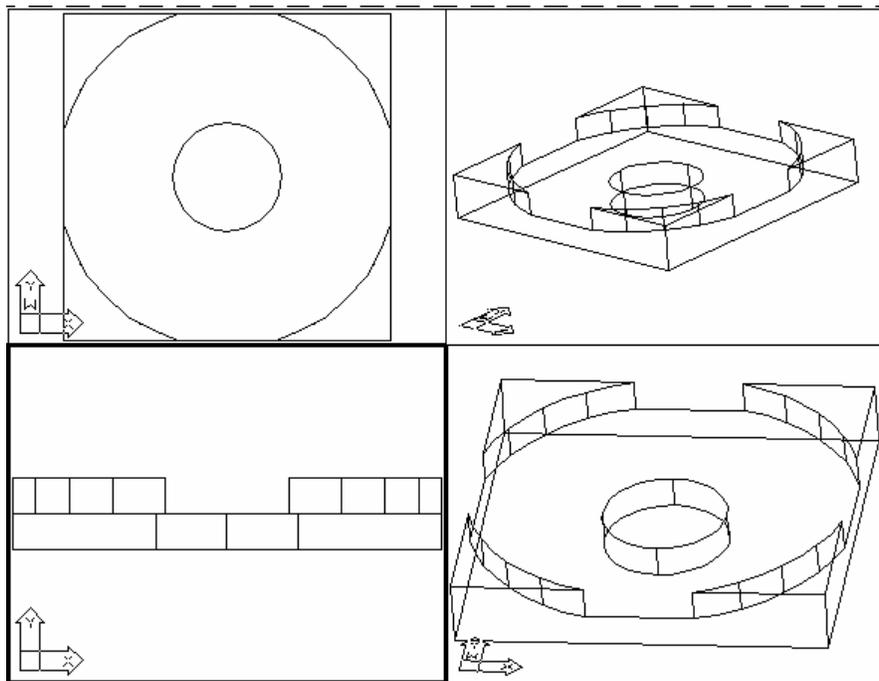
**Fig 8 - Top, left and isometric views of motor mount piece to show how motor sits atop and interacts with the accelerator.**
