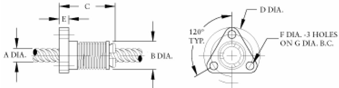
**Figure 1 – A generalized drawing of the lead screw and nut from Kerk Motion.**
