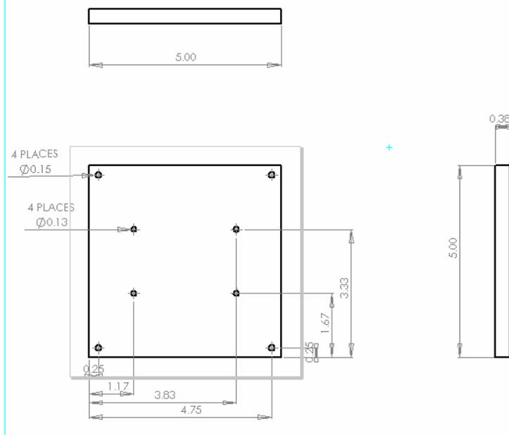
Drawing 3: First Prototype: Stationary Robot Top Plate
