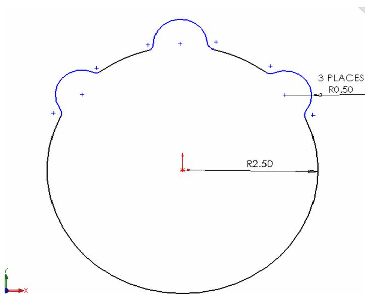
Drawing 6: Final Design – Stationary Robot Base Plate
