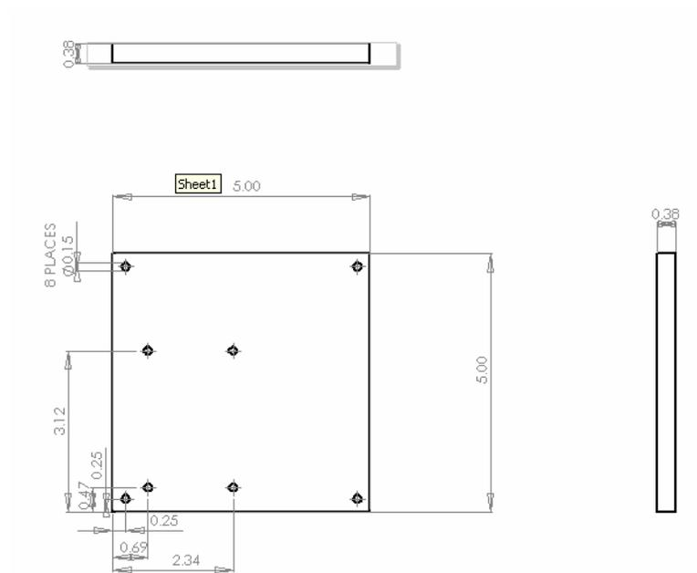
Drawing 2: First Prototype: Stationary Robot Mid Plate
