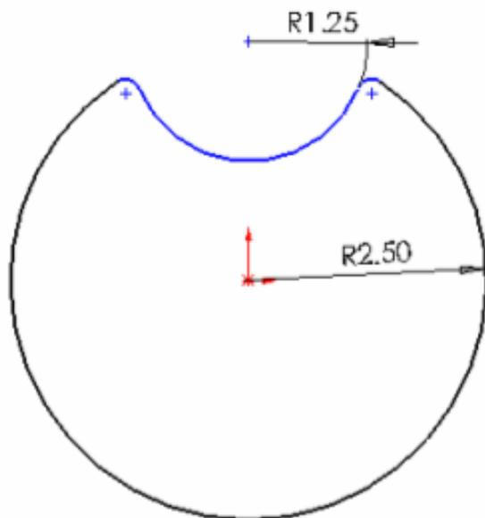
Drawing 7: Final Design –Mid Plate for Stationary Robot
