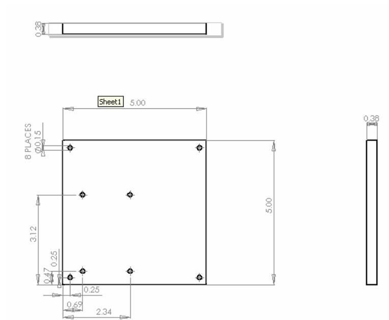
Drawing 1: First Prototype: Stationary Robot Base Plate
