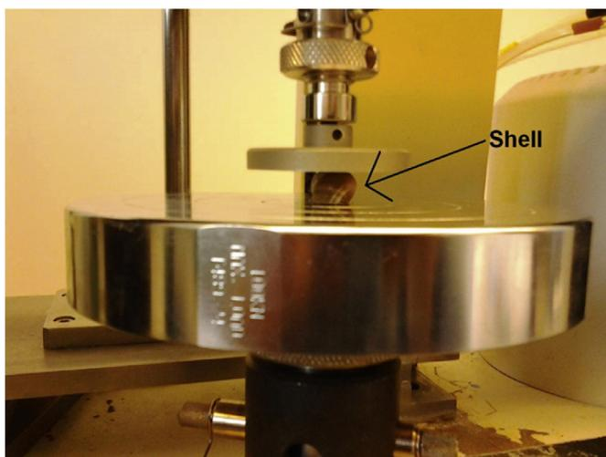
**Fig. 1.** Instron setup for determining breaking force of periwinkle (*Littorina littorea*) shells with and without *Crepidula plana* on the inside. Shells were oriented with the aperture facing downwards, and the crushing surface was projected downward at 1 mm/min.
