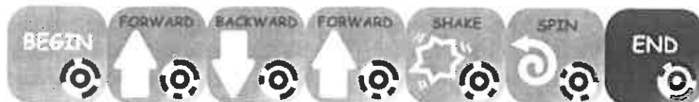
Figure 3. The CHERP program for performing the “Hokey Pokey” dance, as it would appear on the graphical computer interface
