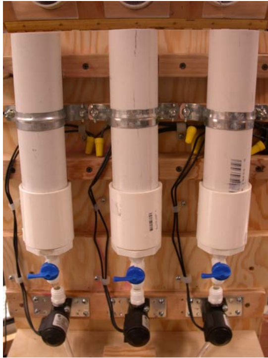
Figure 23: Prototype washing stations with refillable liquid reservoirs & shutoff valves
