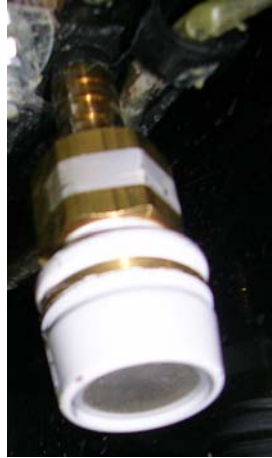
Figure 28: Aerators attached to the dispense tube ends for a desired well wash
