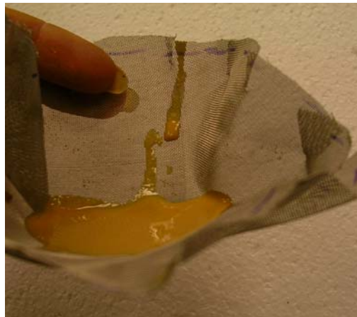
Figure 5: Pure yeast solution exhibited appropriate viscosity to remain on top of wire mesh
