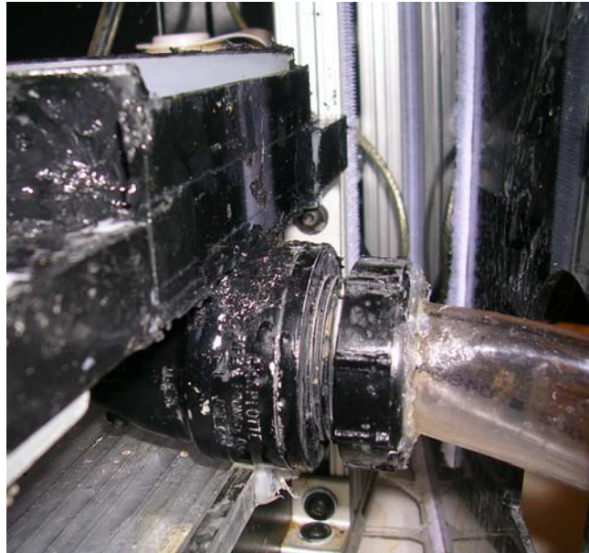
Figure 35: Drainage exit pipe and tube to deposit all excess wash fluid into a separate bucket
