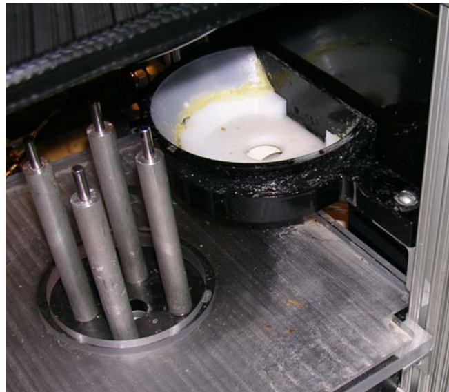
Figure 34: Modified funnel drain to collect excess liquid directly below dispense stations
