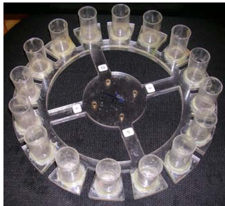
Figure 15: Removal of excess material from well plate to eliminate unwanted liquid pools
