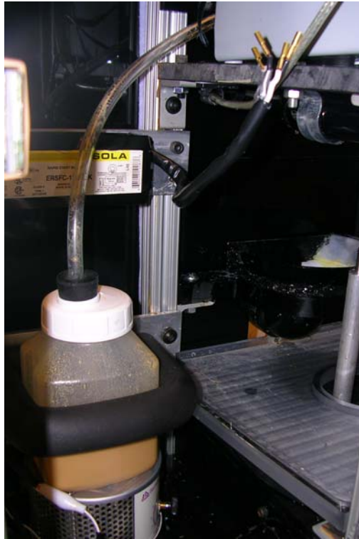
Figure 32: Yeast holding container and magnetic stirrer to maintain a homogenous solution
