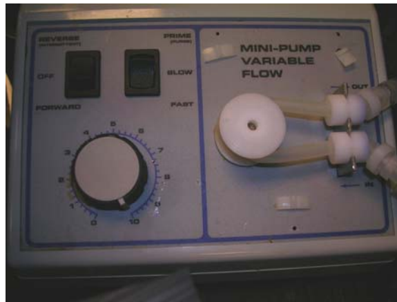
Figure 30: Peristaltic pump to dispense 3.2 mL of yeast solution in each well
