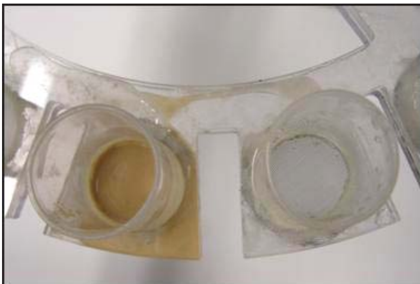
Figure 43: Before (left) and after (right) of pulse-washing
