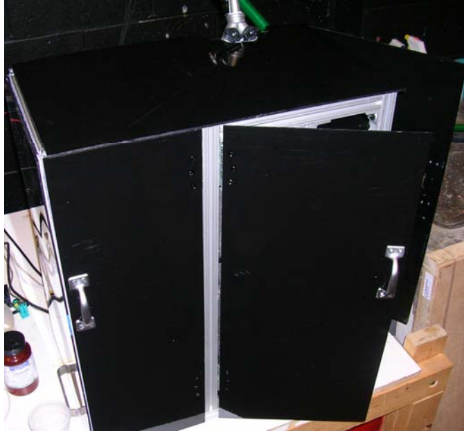
Figure 37: Delrin sheets encase the system to create an appropriate environment for image analysis
