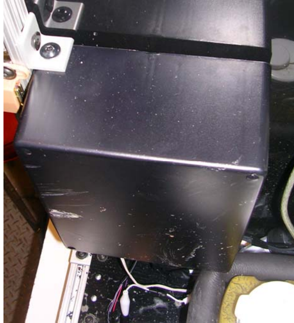
Figure 40: Electrical box mounted in left compartment to house the controller board.
