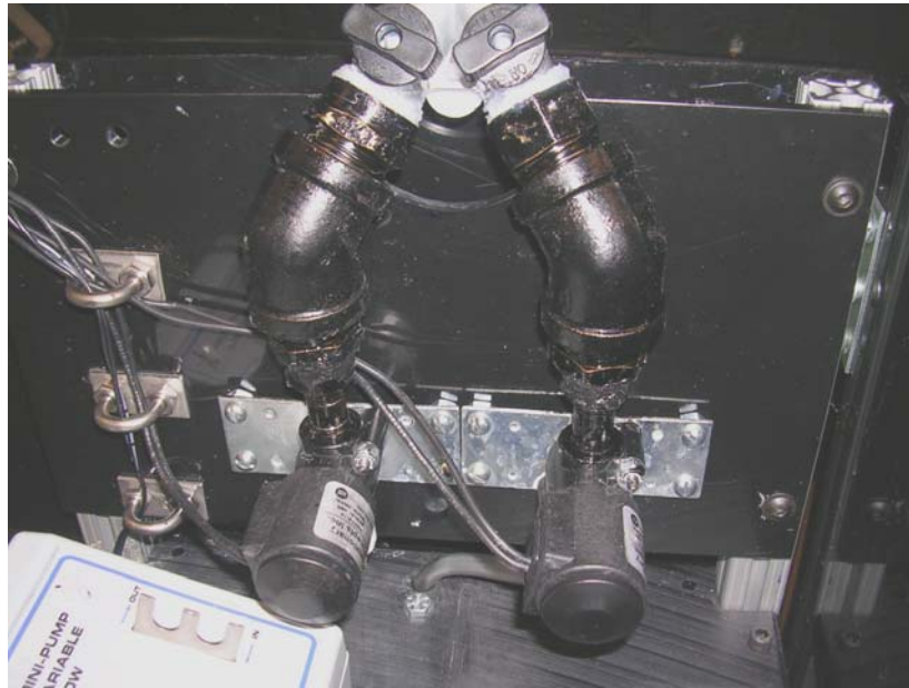
Figure 26: Final valve mount plate secured on the system back frame.
