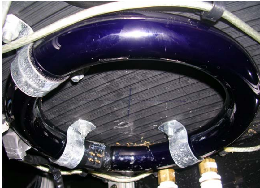
Figure 39: UV light of image processing system mounted to underside of top plate
