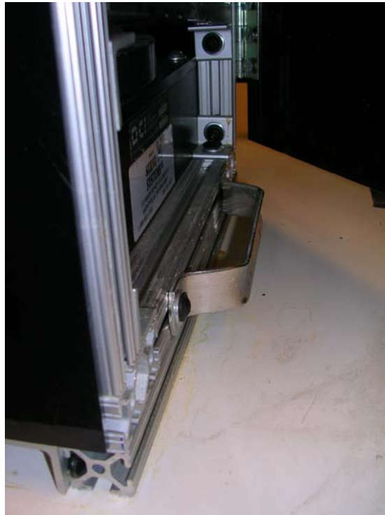
Figure 38: Handles mounted on the right and left sides of 80/20 aluminum base frame
