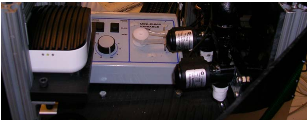
Figure 31: Pump location on top plate is in proximity to washing stations
