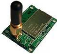
Figure 9: Bluetooth Development Board (Wireless Futures, UK)
