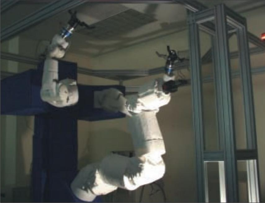
Figure 8. JSC's Cooperative Manipulation Testbed is a three-manipulator system used to prototype and develop advanced control systems for use in space. Control techniques and software developed on CMT enhance the capabilities of systems such as Robonaut.
