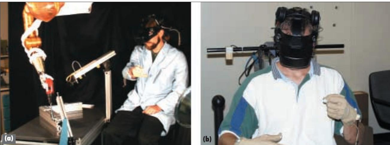
Figure 9. (a) Robonaut under teleoperation and (b) VR gear used to control Robonaut.
