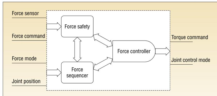
Figure 7. Force controller subautonomy, showing the decision-making, safety, and control processes.
