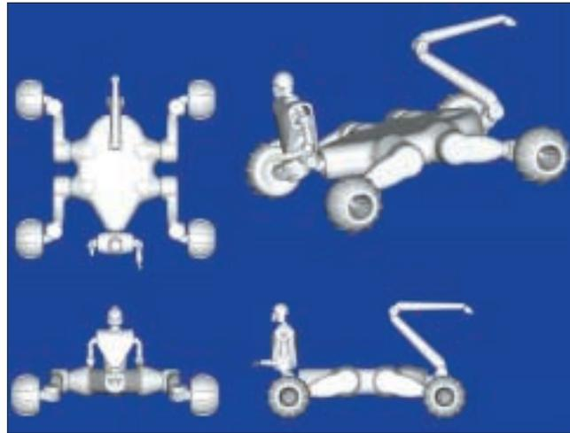
Figure 11. The centaur concept, where the Robonaut attaches to a rover.
