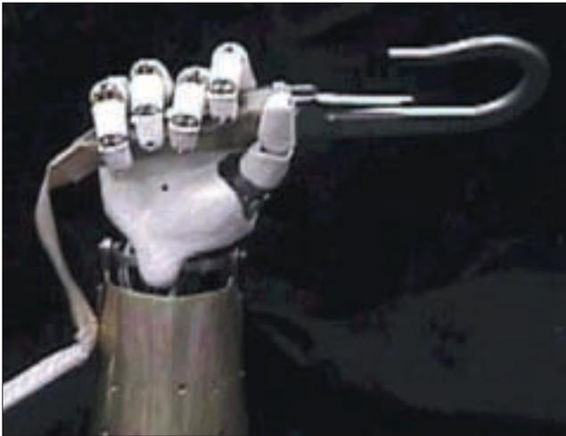
Figure 10. Robonaut unclatching a locking tether hook.
