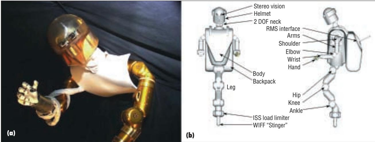
Figure 1. Robonaut's (a) upper body and (b) full anatomy, showing its single leg.
