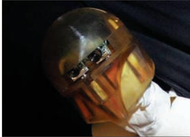
Figure 4. Robonaut head, neck, and camera subsystem.
