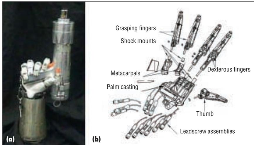
Figure 2. Robonaut's (a) hand, holding a space torque tool; (b) hand parts, showing the dexterous and grasping sets.
