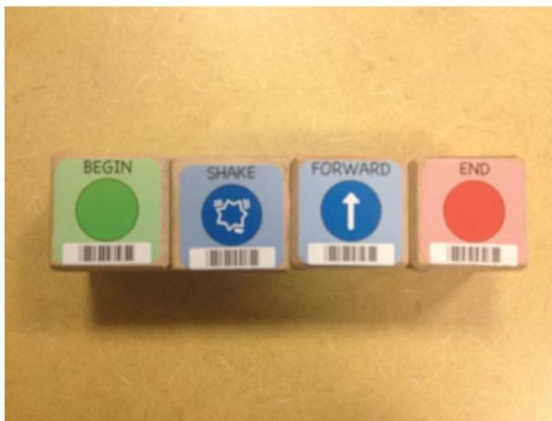
**Figure 2.** Basic program starting with Begin block and finishing with End block.
