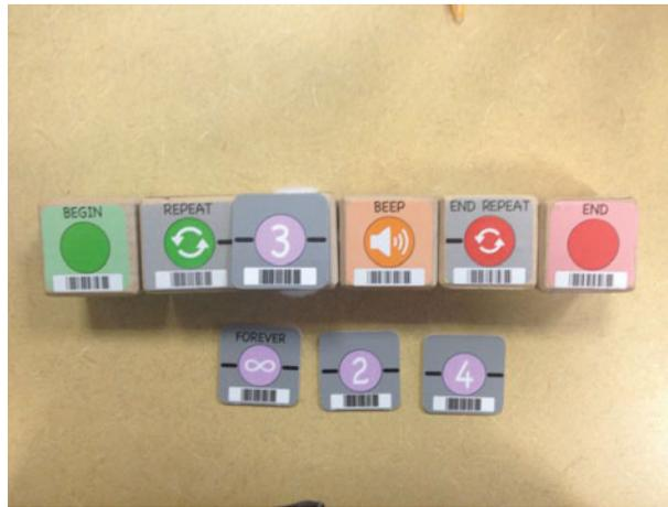
**Figure 3.** Repeat loops program. *Note.* The program above shows a syntactically correct repeat loops program using the number 3 parameter. This program will tell the robot to beep three times. Pictured below the program are choices of other number parameters that can be used for this type of program.
