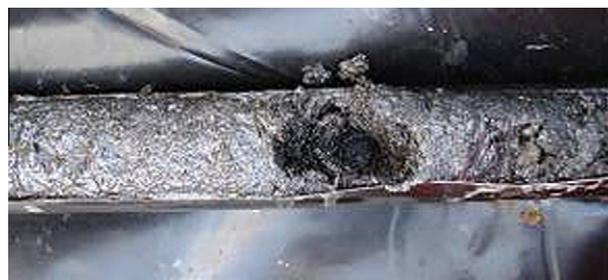
**Fig. 2.** A standard cone penetrometry sampling tube was used to collect coal tar contaminated soil after it was found by the photoionization sensor as the probe was advanced into the subsurface.
