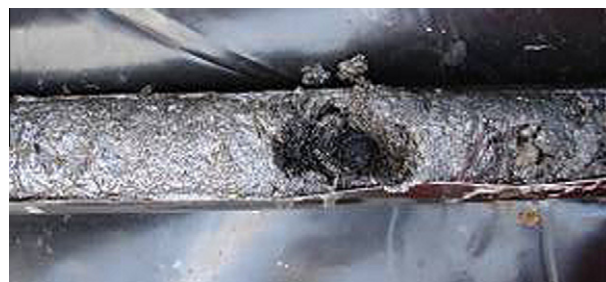
Fig. 2. A standard cone penetrometry sampling tube was used to collect coal tar contaminated soil after it was found by the photoionization sensor as the probe was advanced into the subsurface.
