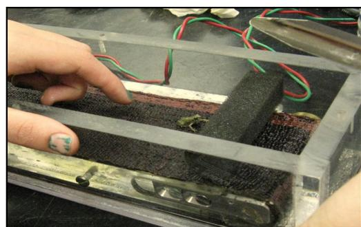
Endurance trials were conducted on a custom-made treadmill and set at a constant speed (.02m/s).
