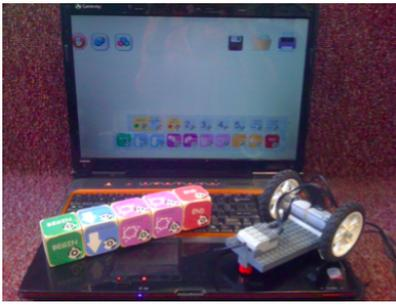
**Figure 1: A sample robot with tangible and graphical interfaces**
